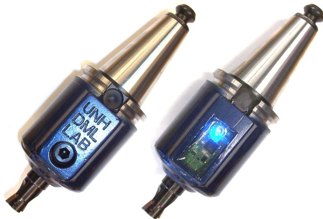
Figure 12. Sensor Integrated Endmilling Tool Fixtured In a Transmitting Tool Holder
