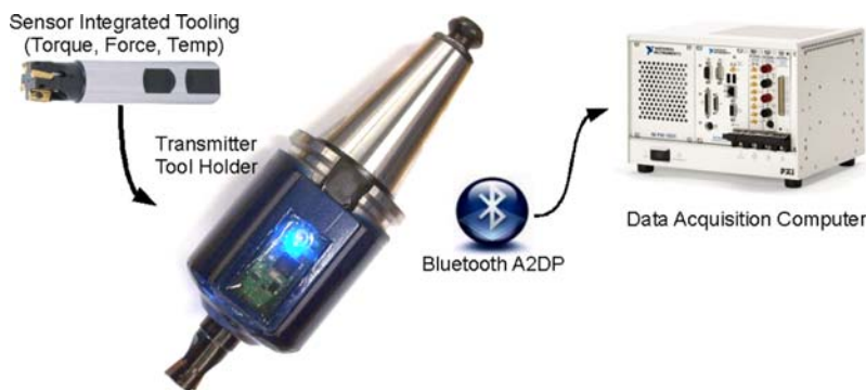
Figure 1 Block diagram of wireless sensor system (see online version for colours)
